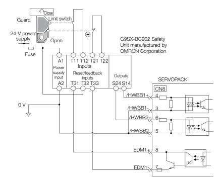
When the guard is opened, both the /HWBB1 and the /HWBB2 signals turn OFF, and the EDM1 signal turns ON. Because the feedback circuit is ON while the guard is closed, the Safety Unit is reset, the /HWBB1 and the / HWBB2 signals turn ON, and the operation is enabled.
