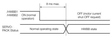
Note: 1. The OFF status is not recognized if the OFF interval of the /HWBB1 or /HWBB2 signal is 0.5 ms or shorter.
